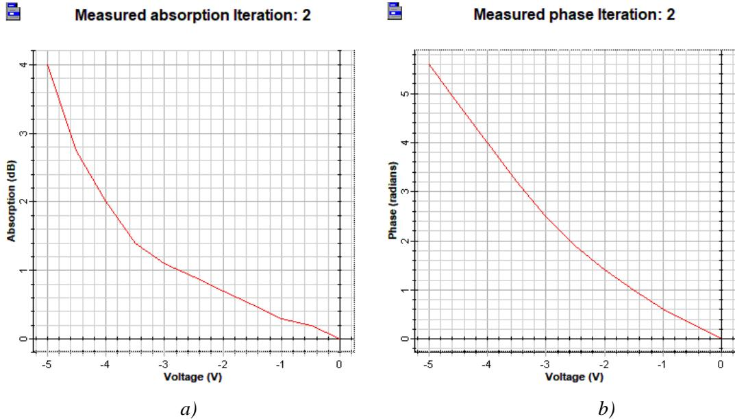
Fig. 3. MZM<sub>1</sub> voltage to absorption curve (a), MZM<sub>2</sub> phase (radiation) to voltage curve (b)
