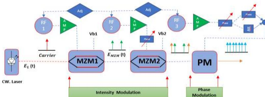
Fig. 2. Three cascades system: MZM<sub>1</sub>, MZM<sub>2</sub> and PM
